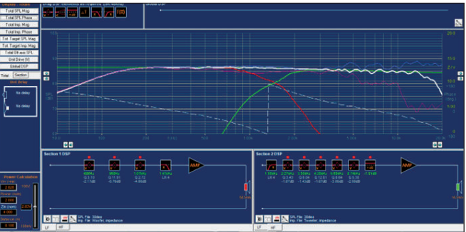
Figure 9: System optimized in FINE DSP using several Biquads. Also, a smoother phase response was achieved (dashed white).
