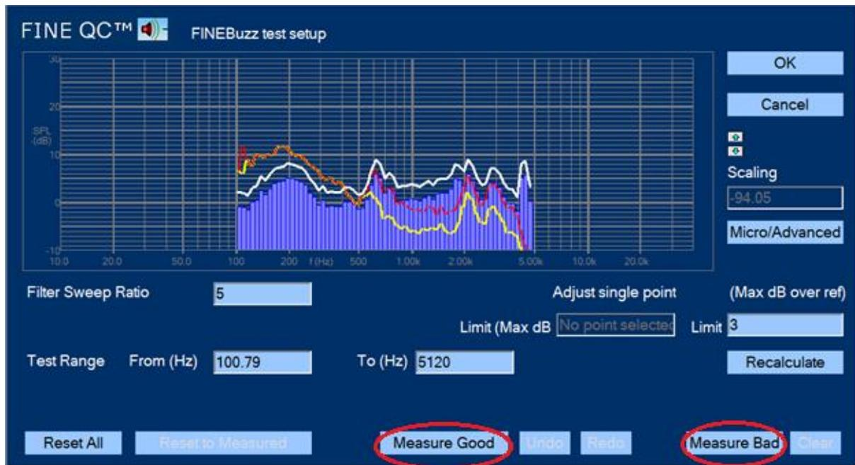
**Figure 17 - The Rub and Buzz limits are defined by measuring some good and some bad drivers. FINEQC will then calculate the limits.**
