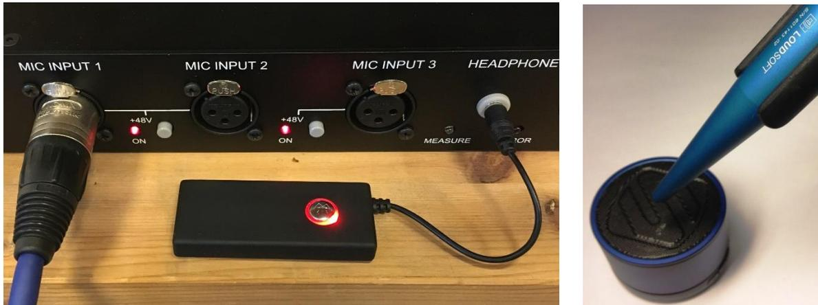
Figure 42 - Bluetooth Transmitter connected to Headphone output
