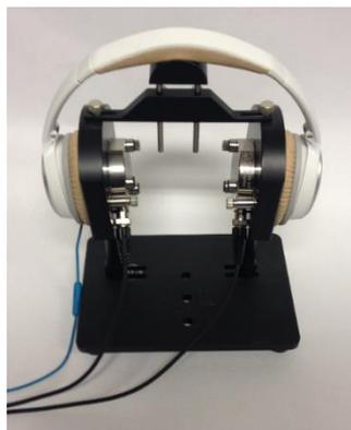
**Figure 34 - CRY Headphone Test Fixture**
