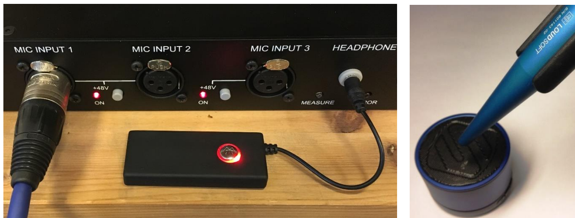
Figure 47 - Bluetooth transmitter connected to Headphone output, which is in parallel with the Line Out.
